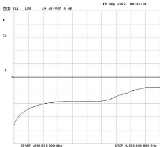
Return loss tested to 6.5 GHz for the CRF Reed Relay. Horizontal full scale: 6.5 GHz. Vertical scale: 10 dB/div referenced from the 0 mark.
