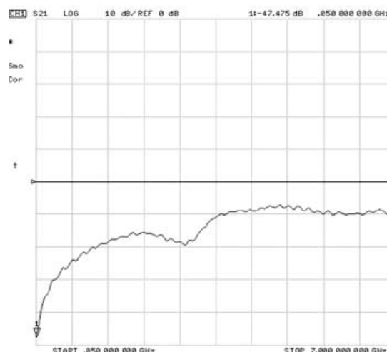
Isolation tested to 7 GHz for the CRF Reed Relay. Horizontal full scale: 7.0 GHz. Vertical scale: 10 dB/div referenced from the 0 mark.
