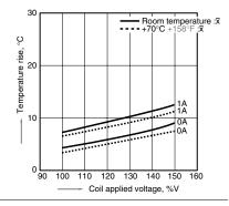
5-(2). Coil temperature rise Tested sample: TXS2-24V, 6 pcs. Point measured: Inside the coil Ambient temperature: 25°C 77°F, 70°C 15
