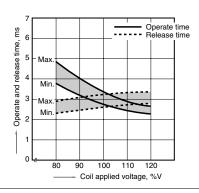
6-(2). Operate and release time (without diode) Tested sample: TXS2-4.5V, 10 pcs.
