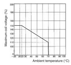
**Note:** The maximum coil voltage refers to the maximum value in a varying range of operating power voltage, not continuous voltage.
