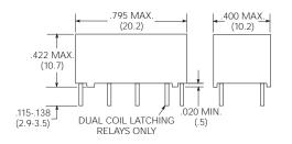
Coil Terminals: 0.015" (.38mm) dia. typical. Contact Terminals: 0.020" (.5mm) x .010" (.25mm) typical. (0.020" dimension is measured in the direction of the .795" dimension of the relay.)
