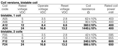
All figures are given for coil without preenergization, at ambient temperature +23°C Other coil voltages on request
