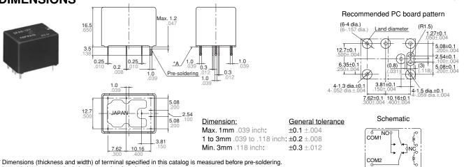
\* Dimensions (thickness and width) of terminal specified in this catalog is measured before pre-soldering. Intervals between terminals is measured at A surface level.
