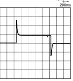
6-(2). Electrical life test (Motor lock) Sample: CF2-12V, 3pcs.
