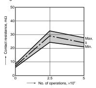
5-(2). Electrical life test (5 A 250 V AC, resistive load) Sample: ALA2PF12, 6 pcs. Operation frequency: 20 times/min. (ON/OFF = 1.5s: 1.5s)Ambient temperature: 20°C 68°F
