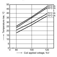
4. Ambient temperature characteristics and coil applied voltage
