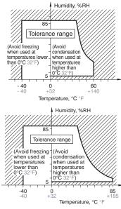
\* -40 to +85°C -40 to +185°F (When 45% to 80%V of coil holding voltage)
