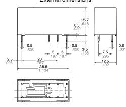
**Dimension:** <u>Tolerance</u> Less than 1mm .039inch: ±0.1 ±.004 Min. 1mm .039inch less than 3mm .118 inch:  $\pm 0.2 \pm .008$ Min. 3mm .118 inch: ±0.3 ±.012
