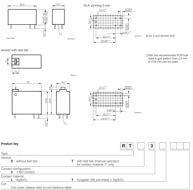
Datasheet Rev. FE1 Issued 2006/05 www.tycoelectronics.com www.schrackrelays.com Dimensions are in mm unless otherwise specified and are shown for reference purposes only. Product specification according to IEC 61810-1. Product data, technical parameters, test conditions and processing information only to be used together with the 'Definitions' at schrackrelays.com in the 'Schrack' section. Specifications subject to
