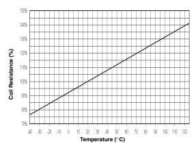
Example: Resistance of  $210\Omega$  coil = 75% of  $210\Omega$  at -40° C, or  $158\Omega$  = 100% of  $210\Omega$  at  $20^{\circ}$  C, or  $210\Omega$  = 125% of  $210\Omega$  at  $85^{\circ}$  C, or  $263\Omega$
