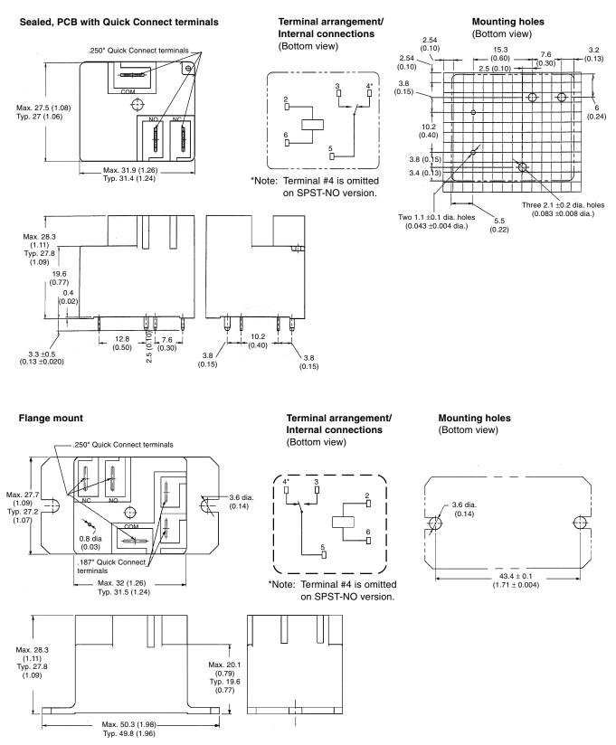
Note: Allow air circulation within the sealed type G8P by removing the ventilation nib from the cover after soldering and cleaning is complete.
