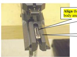
Align the orientation of the connector body and cover assembly.
