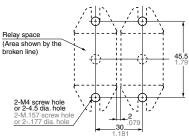
Tolerance:  $\pm 0.1 \pm .004$  (Pitch for side-by-side mounting)
