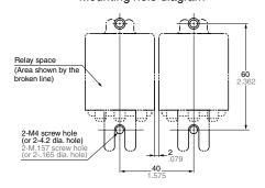
$\label{eq:total_total_total} Tolerance: \pm 0.1 \, \pm .004$  (Pitch for side-by-side mounting)
