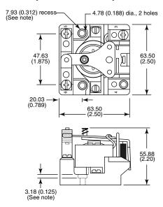
Note: Recess for screw mounting on units with 300-600 VAC coils
