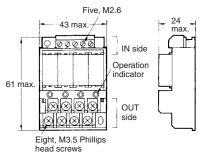
Note: Do not reverse the coil polarity.
