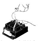
Be sure to turn OFF the power to the Unit before replacing a Relay. Relays must be inserted straight onto the socket connector pins to ensure proper connection.
