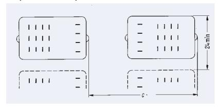
When mounting cradle relay P consideration should be given to magnetic fields. Strong DC magnetic fields, possibly caused by adjacent relays, and large iron masses are the most common causes of interference. Experience has shown that under normal operating conditions the minimum spacings specified for cradle relay P are sufficient to prevent cross interference.
