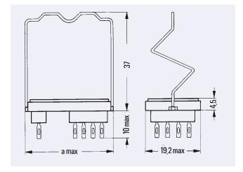
with hold-down spring for cradle relay W
