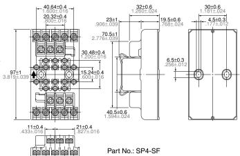
Note: Terminal number marking is on the socket body. Please refer together with the SP relay schematic.
