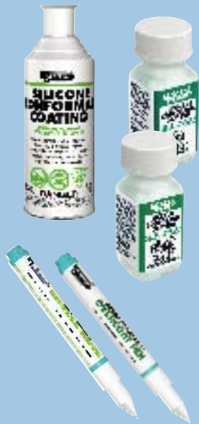
Conformal Coatings are most commonly used. They are easy to apply and very effective at preventing your PCB from corroding, short circuiting, or arcing. Simply clean your board and spray or brush the product on. You will be left with a board that is coated with a transparent coating of approximately 1 mil thick (one coating).
