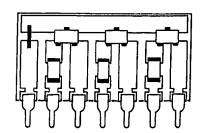
In the example above a transistor array is shown assembled on a standard Surfboard. The mounting zones for the bias resistors were created with the simple technique shown at left. The common buss for the transistor collectors is connected to pin 1 with a jumper.
