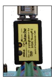
When you connect the Stache to a good 9 volt battery, the green light will flash briefly. Plug the Stache into the programming connector on your Stamp project or carrier board. Refer to the box if you do not have a standard connector and need to construct an adapter. Be sure the power to your project is also turned on—the Stache battery does not power your Stamp
