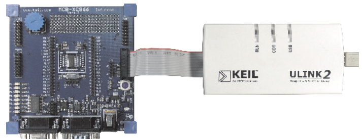
The Keil ULINK2 Debug Adapter connects to a wide range of evaluation boards. For more information refer to www.keil.com/ulink
