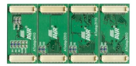
The kit contains two 44-pin TQFP adapters, two 8-pin SOIC adapters, two 20-pin SOIC adapters and two 44-pin PLCC adapters.
