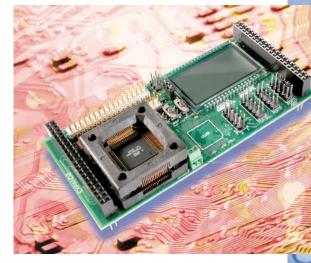
The STK502 demonstrates all the capabilitie of the Low Power ATmega169 AVR® Flash microcontroller. Two applications notes designed to run on the STK502 hardware help reduce time-to-market for designers using the ATmega169.
