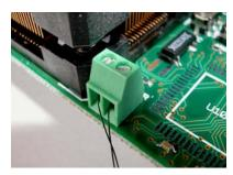
STK502 supports both the In-System Programming mode and the High-voltage Programming mode. AVR Studio, Atmel's front-end tool for the STK500 Development Board, provides support for STK502.
