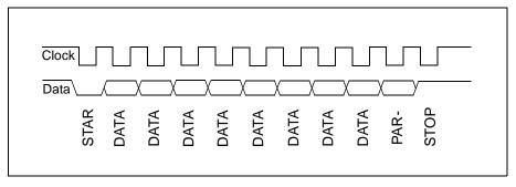
Figure 2.2: Device-to-Host Communication (Data bit Read on Falling Edge of Clock)
