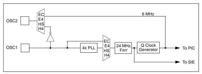
Figure 3.1: Oscillator/PLL Clock Control
