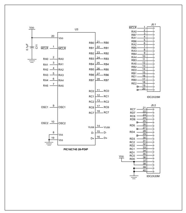
Figure A.3: PIC16C745 and Expansion Connector
