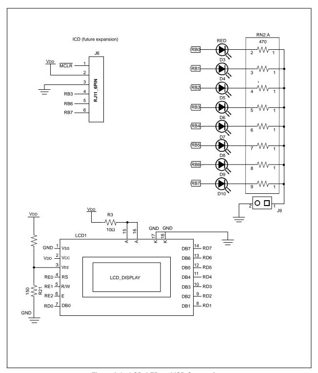
Figure A.2: LCD, LED and ICD Connections
