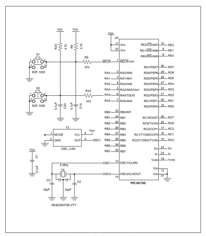
Figure A.4: PIC16C765 and Oscillator
