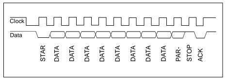
Figure 2.3: Host-to-Device Communication (Data bit Read on Rising Edge of Clock)
