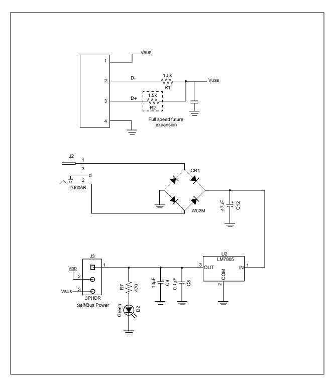
Figure A.5: Power Supply and USB Connections
