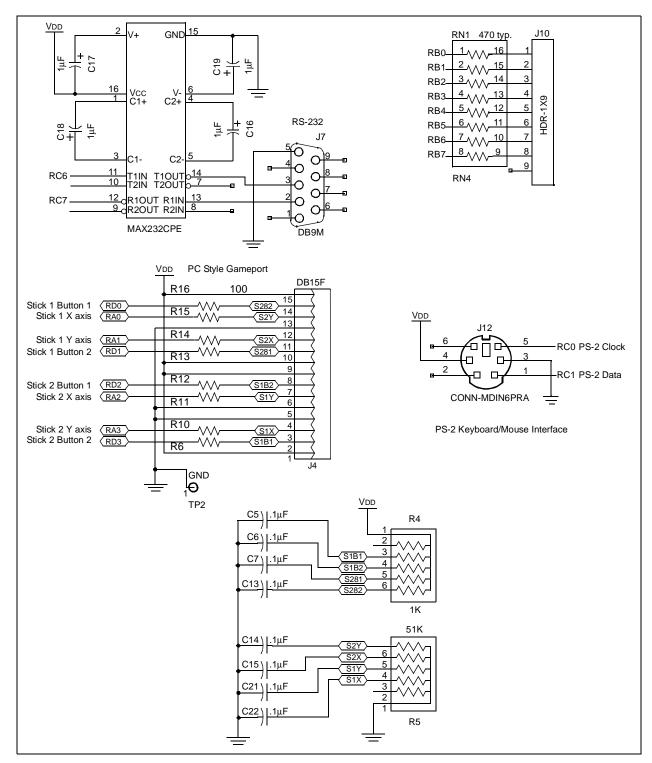
Figure A.1: PC Peripheral Connectors
