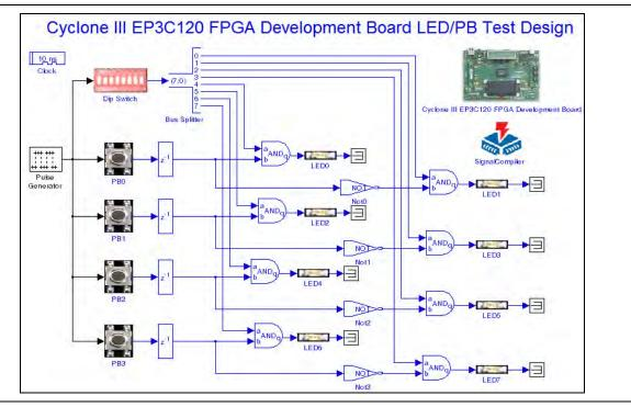
Figure 11-6. LED and Push-button Design Example for the Cyclone III EP3C120 DSP Board Blocks
