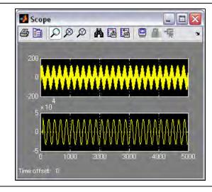
Check that the FIR filter block behaves as you expect and filters high-frequency data as a low-pass filter.
