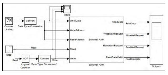
Figure 8–1. External RAM Block Example
