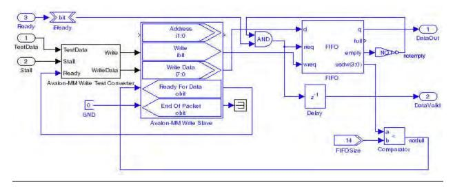
The Avalon-MM Write Test Converter block handles caching and conversion of Simulink or MATLAB data into accesses over the Avalon-MM interface. You can use this block to test the functionality of your design. The Avalon-MM Write Test Converter is simulation only and does not synthesize to HDL.
