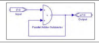
To avoid this error, include an AltBus block configured as an internal node to specify the bit width in the feedback loop explicitly (Figure 13–2).
