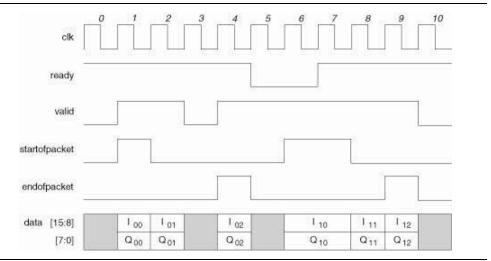
The *Avalon Interface Specifications* also describe several mechanisms to support the transfer of data associated with multiple channels. Altera recommends that you achieve this mechanism with packet based transfers where each packet has a deterministic format and each channel is allocated a specific field (time slot in a packet).
