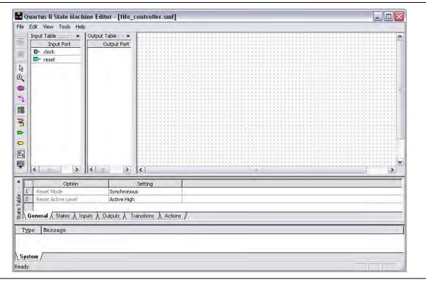
3. On the Tools menu in the Quartus II State Machine Editor, point to **State Machine Wizard** and click **Create a new state machine design**.
