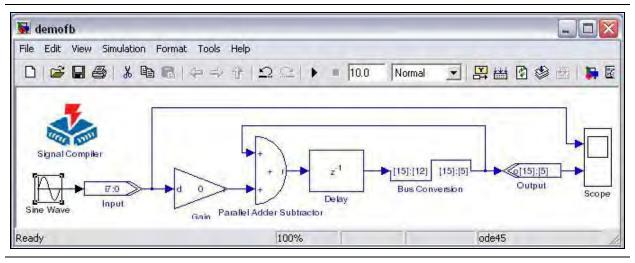
Use the PLL block and assign different sampling periods on registered DSP Builder blocks to design multirate designs.
