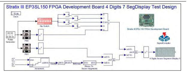
Figure 11–17. 7-Segment Display Design Example for the Stratix III EP3SL150 DSP Board Blocks
