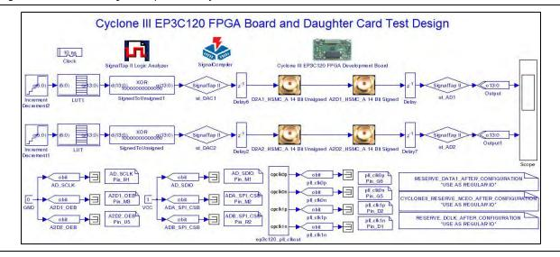
Figure 11-8. HSMC Design Example for the Cyclone III EP3C120 DSP Board Blocks
