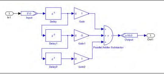
The **fir3tapsub.mdl** design is a 3-tap finite impulse response (FIR) filter and has the following attributes:
