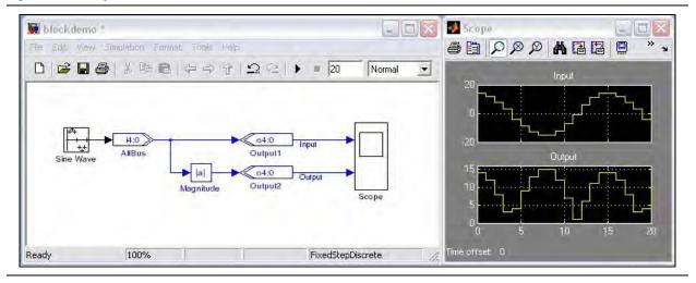
The Magnitude block translates as a combinational signal in VHDL. DSP Builder does not add clock pins to this function.
