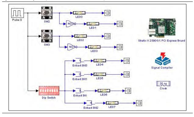
Figure 11–15. Design Example for the Stratix II EP2S90GX PCI Express Board
