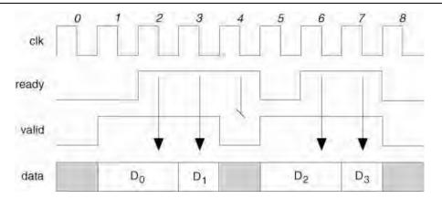
Figure 7–12. Avalon-ST Interface Timing for ready-latency=0
