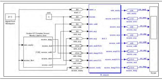
Figure 5–7. DSP Builder Design Using the FFT MegaCore Function
