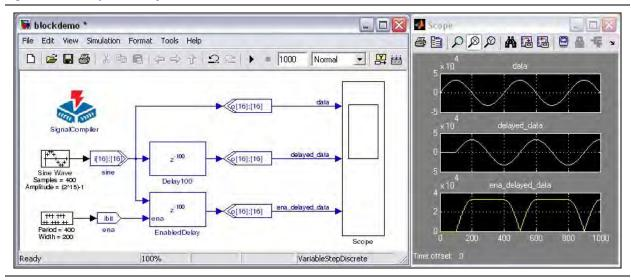
For feedback circuitry (the output of a block fed back into the input of a block), a registered block must be in the feedback loop. Otherwise, DSP Builder creates an unresolved combinational loop (Figure 3–13).
