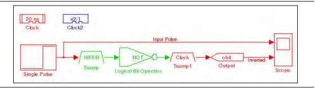
Two DSP Builder blocks can operate with two different sampling periods. However for most DSP Builder blocks, the sampling period of each input port and each output port must be identical.
