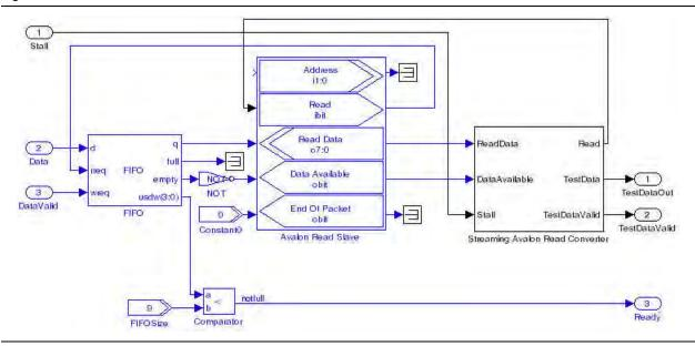
The Avalon-MM Read Data Converter block handles caching and conversion of Simulink or MATLAB data into accesses over the Avalon-MM interface. You can use this block to test the functionality of your design. The Avalon-MM Read Data Converter is simulation only and does not synthesize to HDL.
