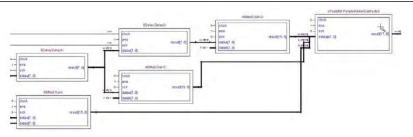
This design requires three multipliers and one parallel adder. The arithmetic operations increase the bus width in the following ways:
