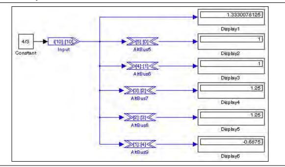
Figure 6–2 illustrates the usage of AltBus to convert a 20-bit bus with a ([10].[10]) signed binary fractional format to a 4-bit bus with a [2].[2] signed binary fractional format.
