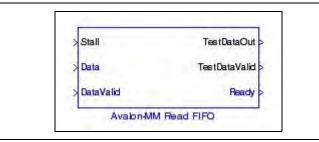
Figure 5–7 shows the content of the  $\ensuremath{\mathsf{Avalon}}-\ensuremath{\mathsf{MM}}$  Read FIFO block.
