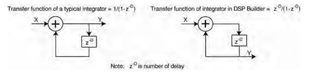
The magnitude response of these two functions is the same although their phase response is different. For the typical integrator function,  $1/(1-z^{-D})$ , there is an impulse on the output at time = 0, whereas the output delays by a factor of *D* for the  $z^{-D}/(1-z^{-D})$  function that the DSP Builder integrator uses.
