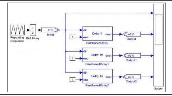
The RamBasedDelay block that **top.mdl** uses, is an example of a custom parameterizable Simulink block. The library file **MyLib.mdl** defines it. The RamBasedDelay block has one parameter, **Delay**.
