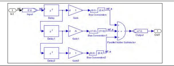
In Figure 3–6, the output of the Gain block has 4 bits removed. Port data type display is enabled in this example and shows that the inputs to the Delay blocks are of type INT\_8 but the outputs from the Bus Conversion blocks are of type INT\_6.
