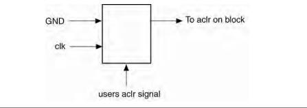
A design may not match the hardware if an asynchronous clear performs during simulation because the aclr cycle may last several clocks - depending on clock speed and the device.
