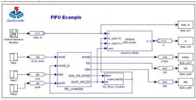
The state machine in this design example feeds the control inputs of a Dual-Port RAM block and the inputs of an address counter.
