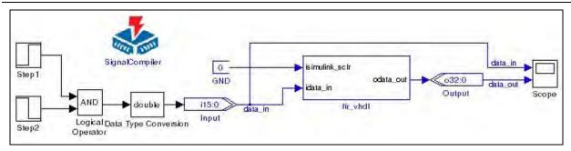
8. Double-click on the fir\_vhdl symbol. The filter8tap/fir\_vhdl subsystem opens (Figure 8–7).
