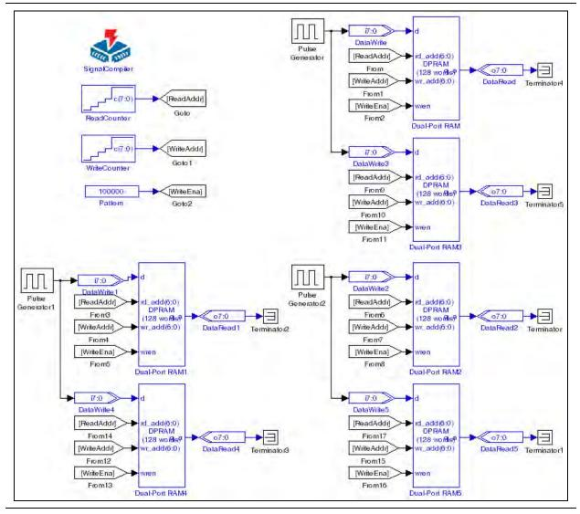
Use the Goto blocks ([ReadAddr], [WriteAddr], and [WriteEna] with the From blocks ([ReadAddr], [WriteAddr], and [WriteEna], which connect to the dual-port RAM blocks.
