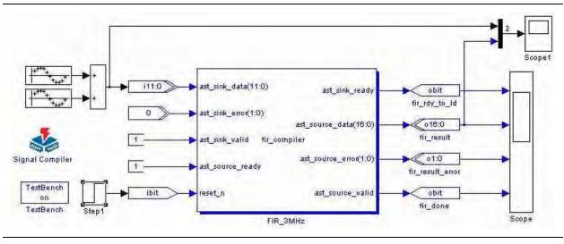
You must simulate an initial reset cycle (with the step input) to replicate hardware behavior. As in hardware, this reset cycle must be sufficiently long to propagate through the core, which may be 50 clock cycles or more for some MegaCore functions such as the FIR Compiler.
