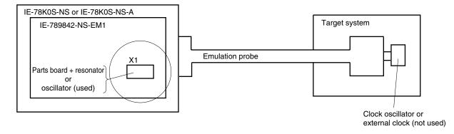
**Remark** The clock that is supplied by the resonator of the IE-789842-NS-EM1 (encircled in the figure) or the oscillator is used.
