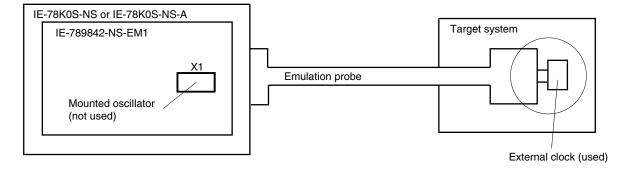
**Remark** The pulse that is supplied by the external clock on the target system (encircled in the figure) or the oscillator is used.
