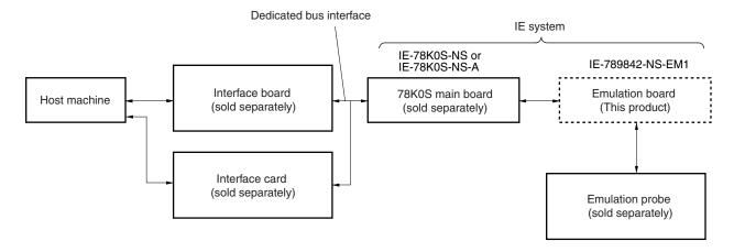
Figure 1-2. Basic Hardware Configuration
