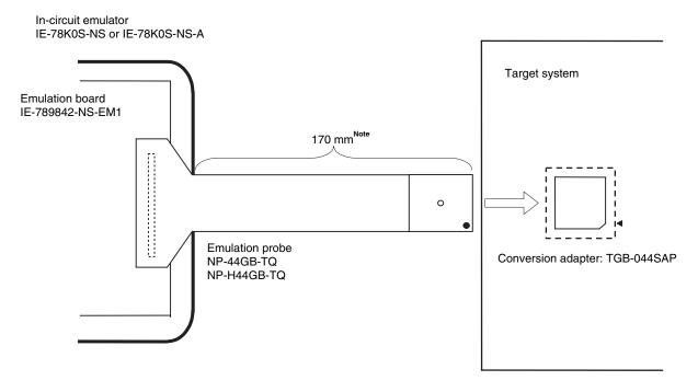
**Note** The above distance shows when the NP-44GB-TQ is used. When the NP-H44GB-TQ is used, the distance is 370 mm.
