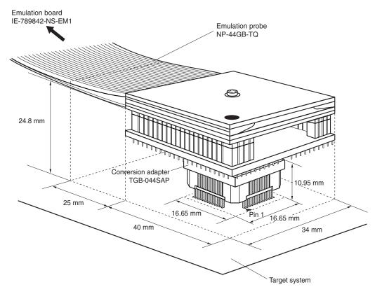
Figure B-2. Connection Conditions of Target System (NP-44GB-TQ)
