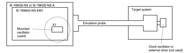
**Remark** The clock that is supplied by the oscillator of the IE-789842-NS-EM1 (encircled in the figure) is used.
