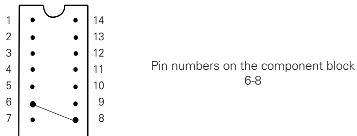
Fig. 4-15 Wiring of Component Block (to use an external clock as the subsystem clock)
