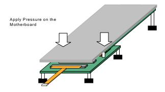
5. Replace the screws on the bottom of the daughterboard to securely connect it to the motherboard (Figure 7).
