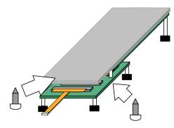
6. Connect the loose end of the probe or ribbon cable to the user target. Refer to Table 2 and Table 3 for pin assignments.
