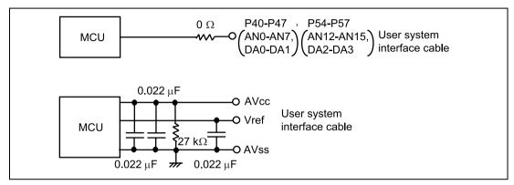
Figure 2.4 User System Interface Circuit for P40 to P47, P54 to P57, Vcc, AVcc, AVss, and Vref Signals
