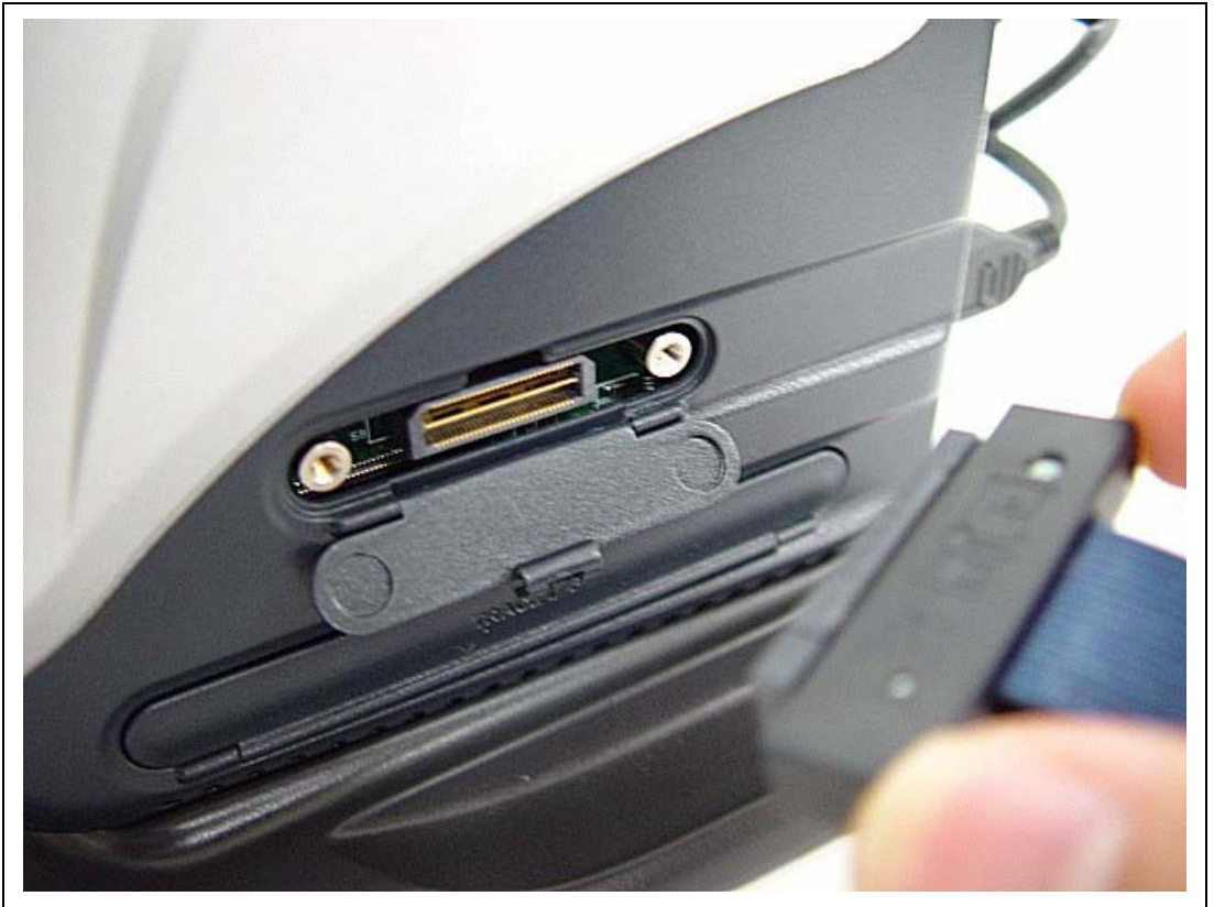
Figure 2.5 Connecting the Analyzer Cable to E200F when Using the Peripheral I/O Analyzer Unit
