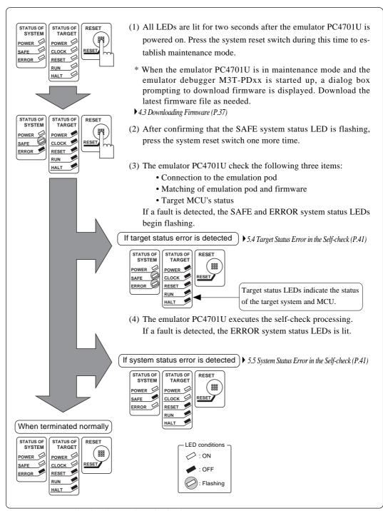
Figure 4.10 LED display during the self-check
