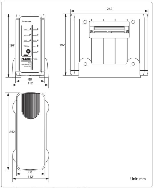
Figure 7.2 External dimensions of the emulator PC4701U
