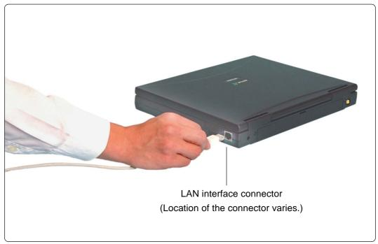
Figure 4.3 Connecting LAN interface cable (host machine side)
