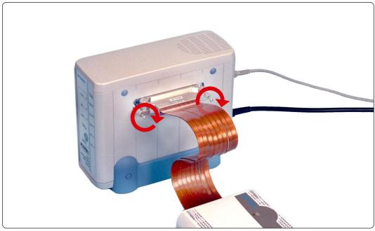
Figure 4.9 Connecting emulation pod
