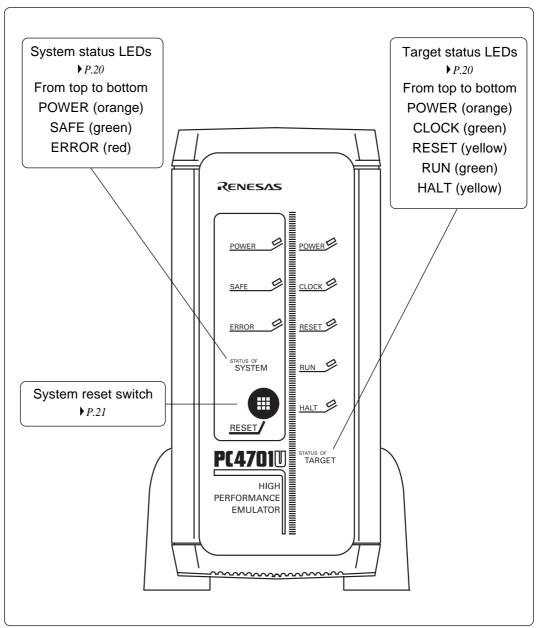
Figure 3.1 Front panel of the emulator PC4701U
