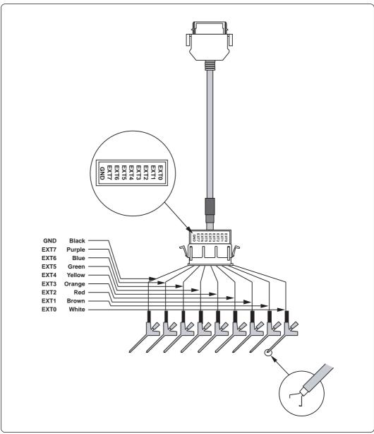
Figure 3.6 External trace signal input cable
