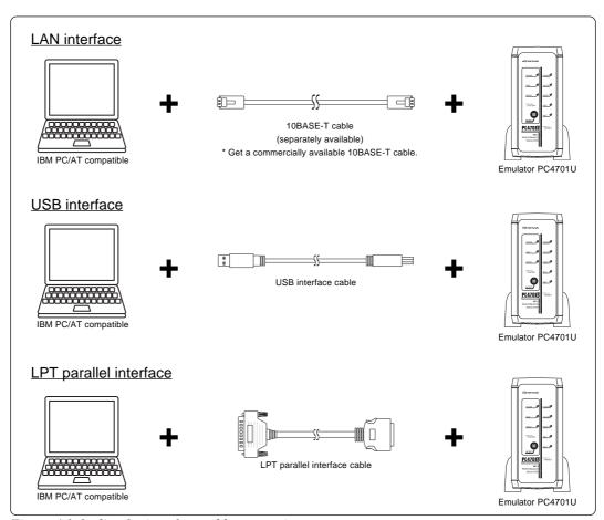
Figure 4.1 Outline for interface cable connection
