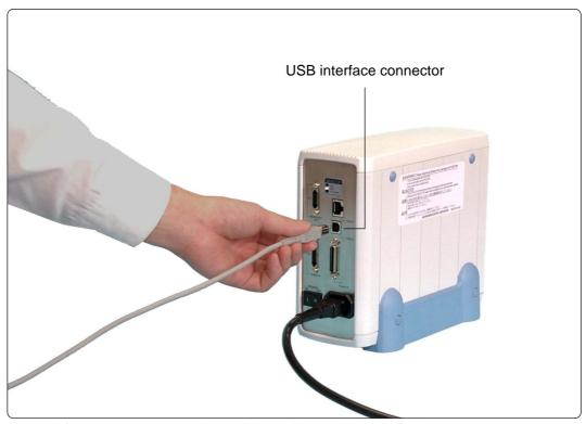
Figure 4.6 Connecting USB interface cable (emulator PC4701U side)
