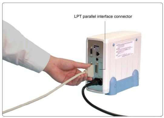
Figure 4.8 Connecting LPT parallel interface cable (emulator PC4701U side)
