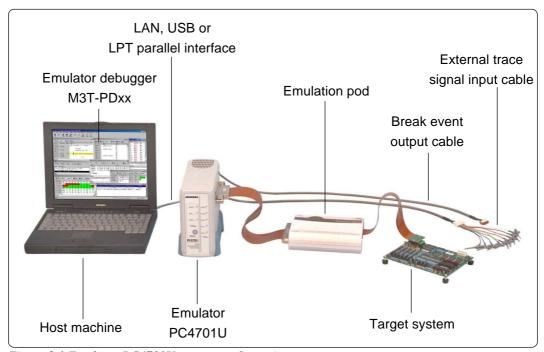
Figure 2.1 Emulator PC4701U system configuration
