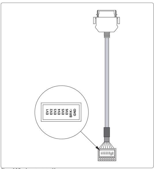
Figure 3.5 Break-event output cable
