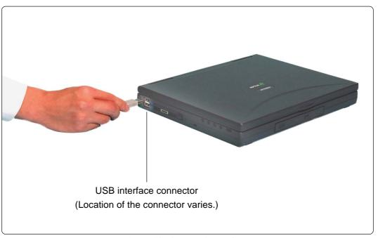
Figure 4.5 Connecting USB interface cable (host machine side)
