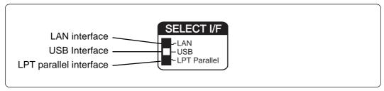
Figure 3.4 Relationship between interface selection switch and interfaces
