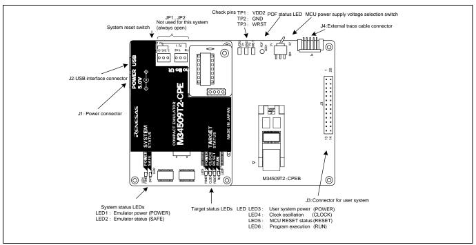
Figure 1.2 Names of the LEDs on the upper panel of the M34509T2-CPE
