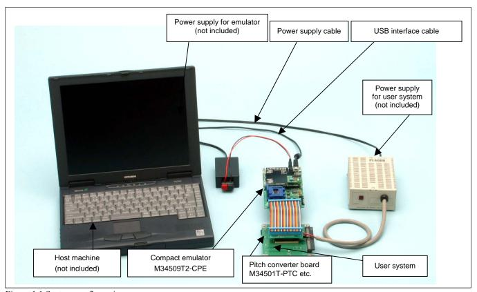
Figure 1.1 System configuration
