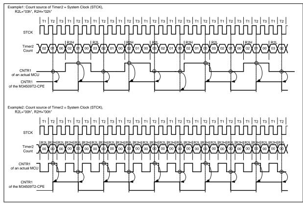
Figure 4.3 Timing of the timer output
