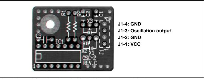
Figure 2.13 External view of the oscillator circuit board OSC-2 and its connector pin locations
