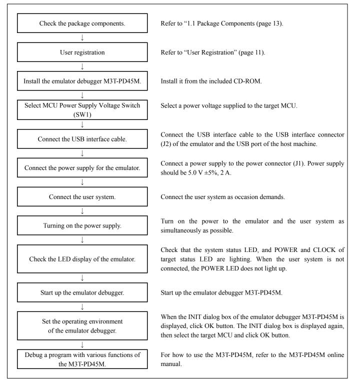
Figure 2.1 Flowchart of starting up the emulator
