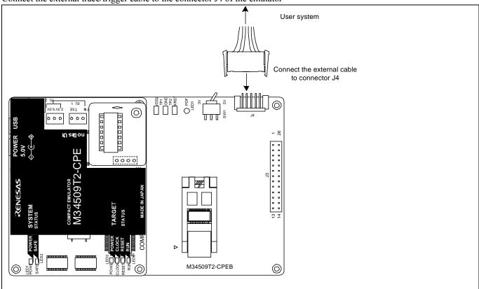
Figure 2.15 Connecting the external trace/trigger cable
