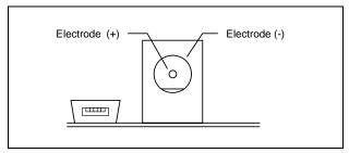
Figure 2.2 Power connector specifications
