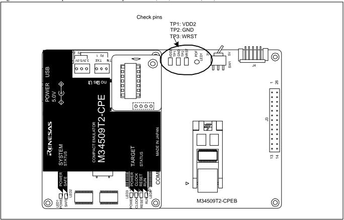
Figure 2.19 Positions of the check pins
