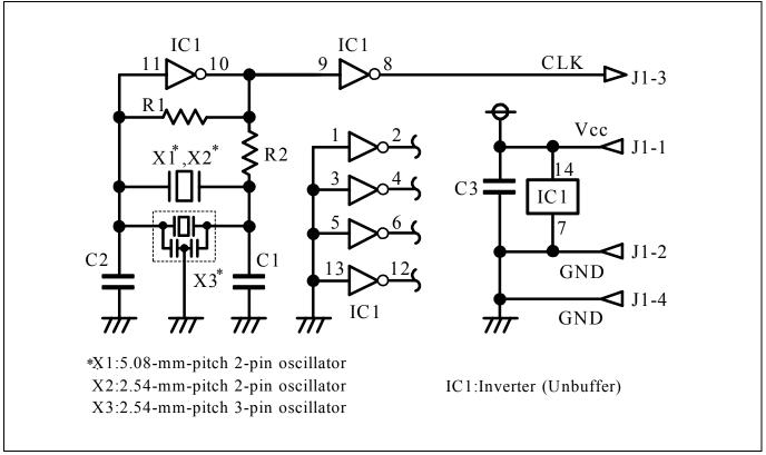
Figure 2.14 Circuits of the oscillator circuit bare board OSC-2
