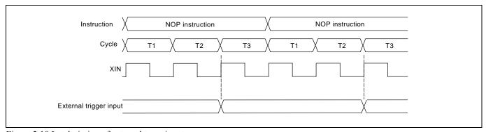
Figure 2.18 Latch timing of external trace input
