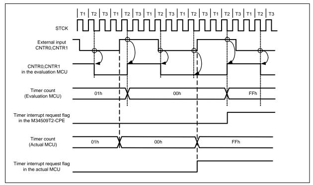
Figure 4.2 Timing of the timer input
