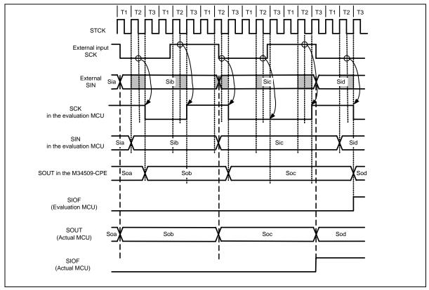
Figure 4.4 Timing of the serial input/output
