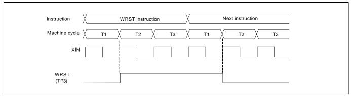
Figure 2.20 Output waveform of the check pin WRST
