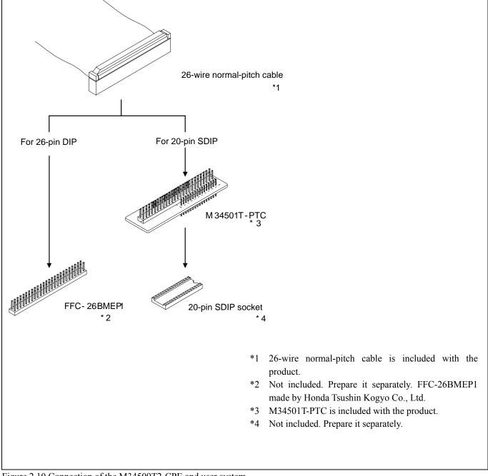
Figure 2.10 Connection of the M34509T2-CPE and user system
