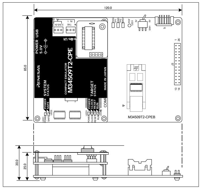
Figure 4.6 External dimensions of the compact emulator
