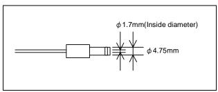
Figure 2.3 Applicable plug specifications
