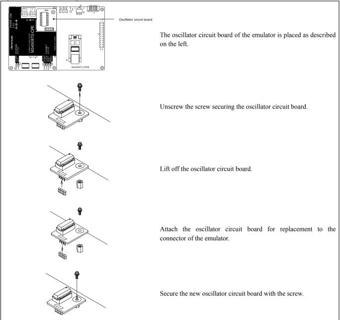
Figure 2.12 Replacing oscillator circuit boards
