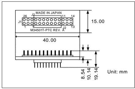
Figure 4.7 External dimensions of the converter board M34501T-PTC
