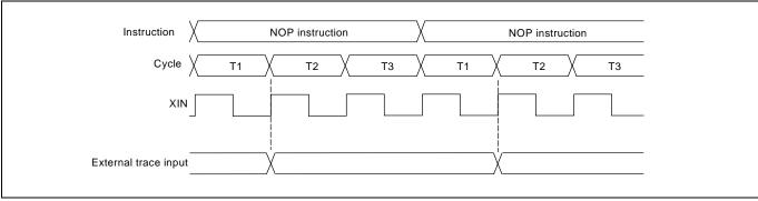
Figure 2.17 Latch timing of external trace input
