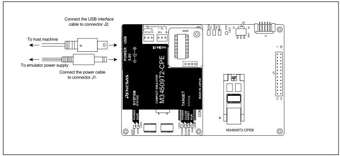
Figure 2.4 Connecting the emulator system
