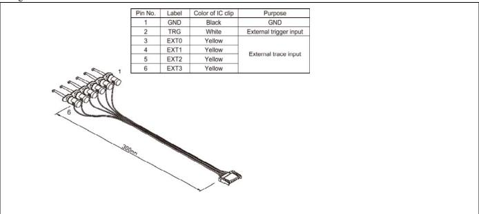
Figure 2.16 Pin assignment of the external trace cable
