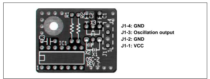
Figure 2.17 External view of the oscillator circuit board OSC-2 and its connector pin locations
