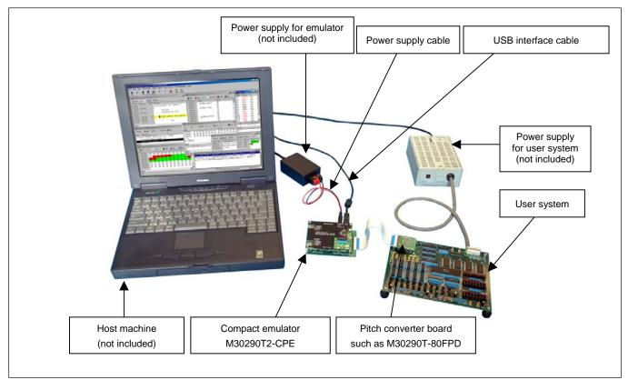
Figure 1.1 System configuration
