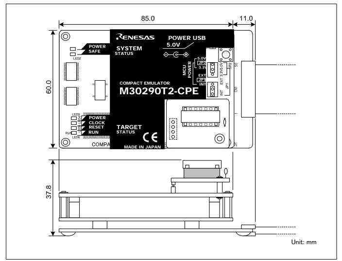
Figure 4.2 External dimensions of the compact emulator
