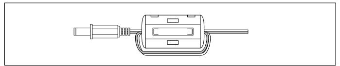
Figure 2.2 Attaching the ferrite core
