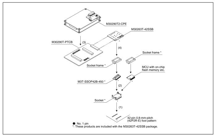
Figure 2.12 Connecting to a 42-pin 0.8-mm-pitch foot pattern
