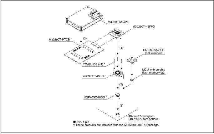
Figure 2.13 Connecting to a 48-pin 0.5-mm-pitch foot pattern
