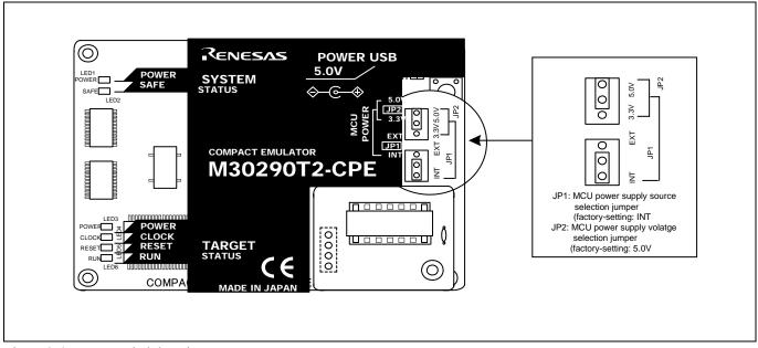
Figure 2.6 Jumper switch locations
