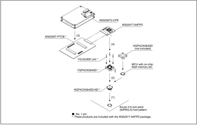
Figure 2.14 Connecting to a 64-pin 0.5-mm-pitch foot pattern
