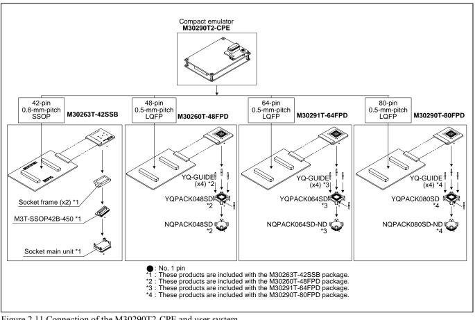
Figure 2.11 Connection of the M30290T2-CPE and user system
