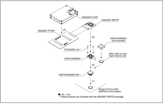
Figure 2.15 Connecting to an 80-pin 0.5-mm-pitch foot pattern
