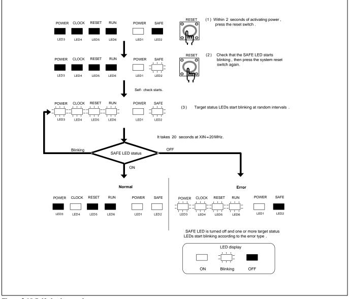
Figure 2.10 Self-check procedure
