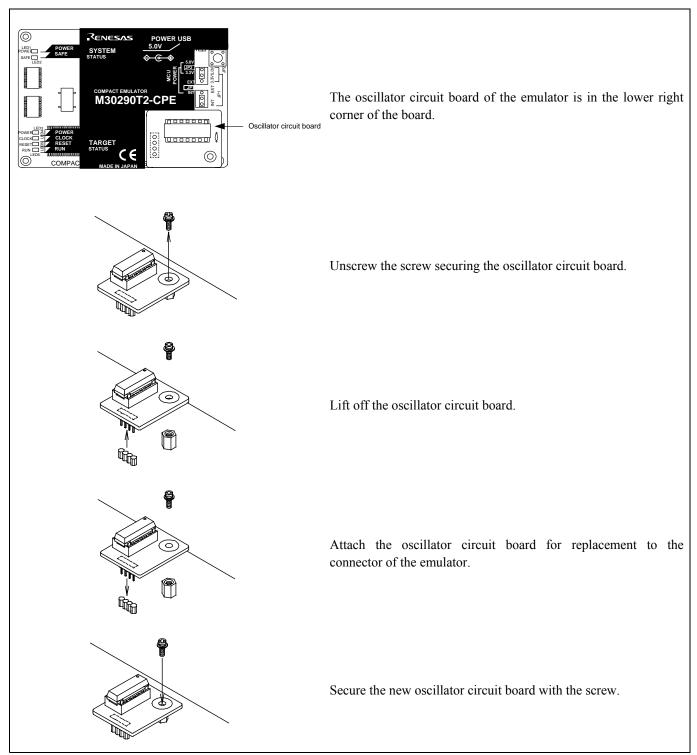
Figure 2.16 Replacing oscillator circuit boards
