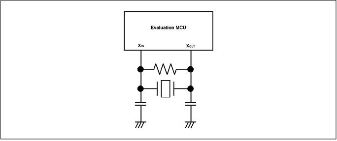
Figure 2.20 Circuit in which oscillation does not occur
