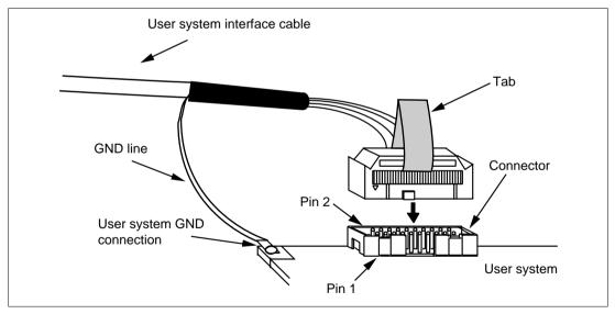
Figure 2.4 Connecting the User System Interface Cable to the User System
