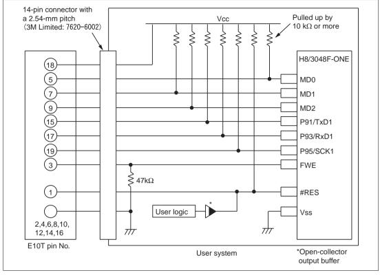
Figure 6.2 Connection of the Emulator (Mode 7)
