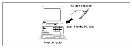
Figure 2.3 Inserting the PCI Card Emulator into the Host Computer
