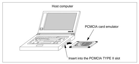
Figure 2.2 Inserting the PCMCIA Card Emulator into the Host Computer
