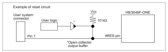
Figure 6.5 Example of Reset Circuits
