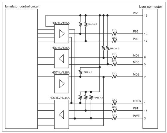
Figure 6.7 Interface Circuit in the Emulator (Reference)
