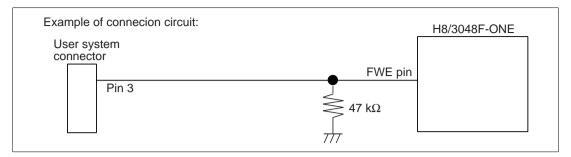
Figure 6.4 Direct Connection of Emulator and FWE Pin
