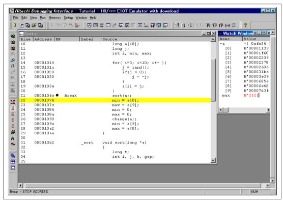
Figure 3.27 [Program] Window (Step Out)
