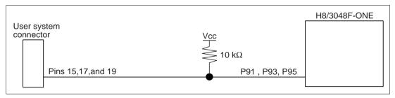
Figure 6.3 Connection of Emulator and P91, P93, and P95 Pin
