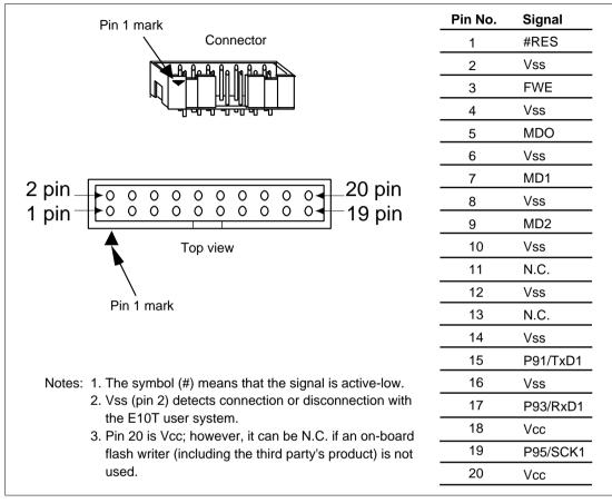
Figure 6.1 Pin Arrangement of the Connector
