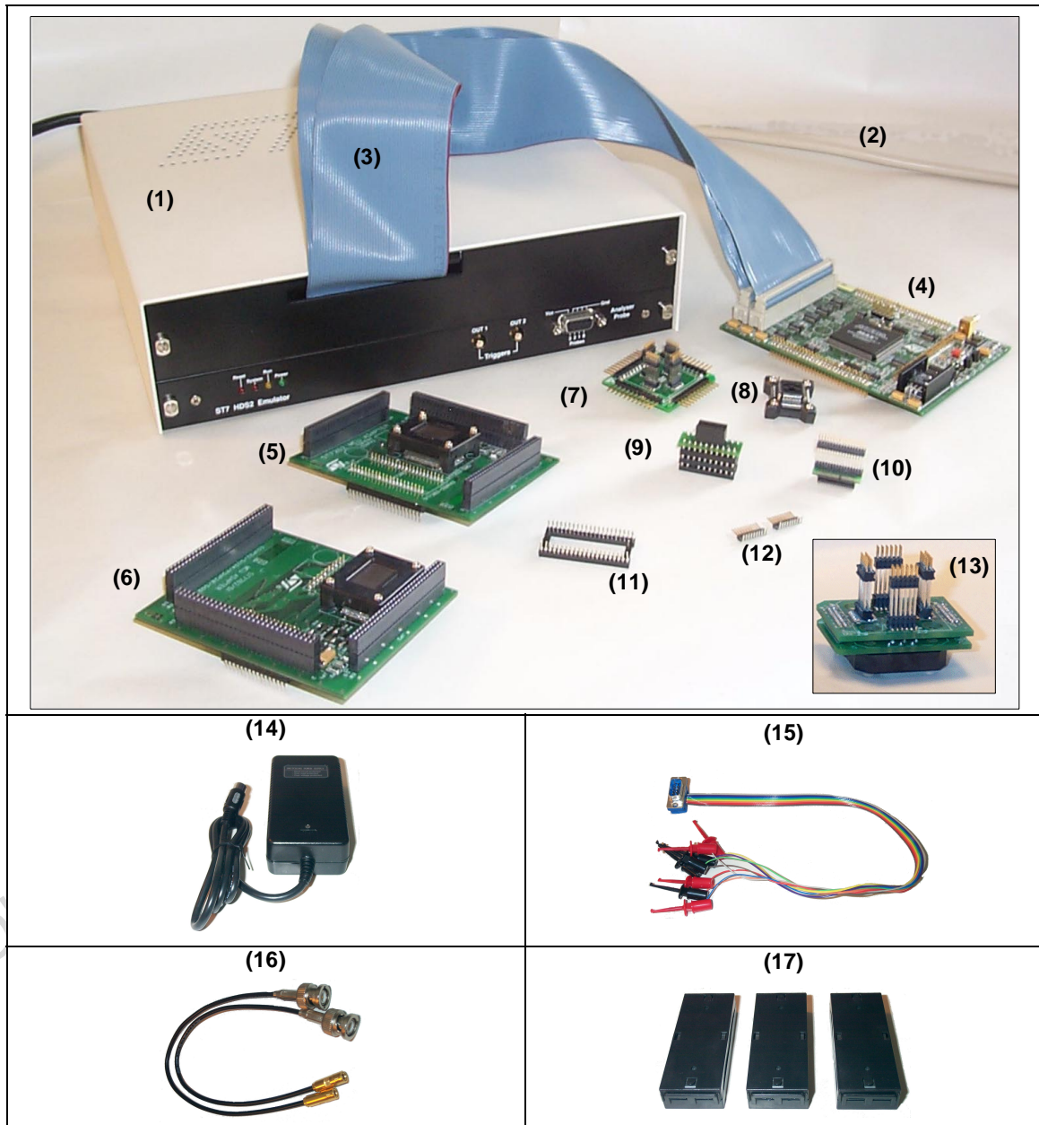
Figure 2: Main components of ST7MDTU2-EMU2B emulator kit
