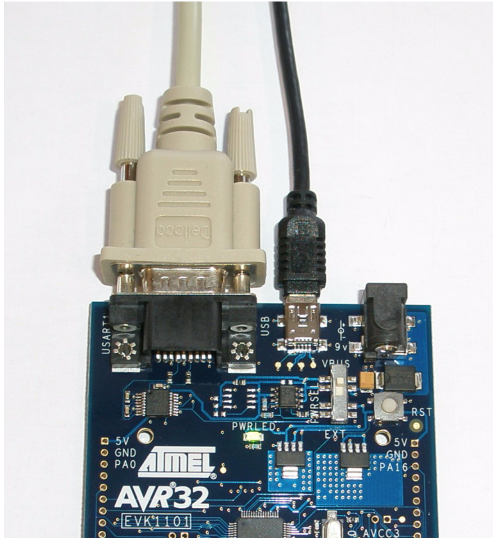
Figure 4-2. Powering the EVK1101 using the USB cable
