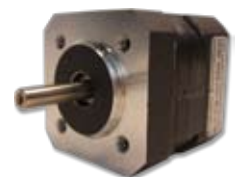
BLDC Motor Anaheim Automation 15V, 8-pole, 8000 RPM Model: bly171s-15v-8000
