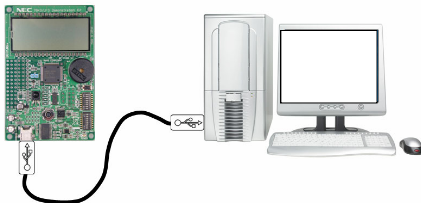
Figure 1. DemoKit-LF3 system configuration
