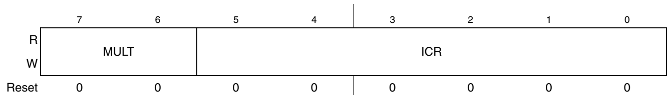
Figure 11-4. IIC Frequency Divider Register (IICF)
