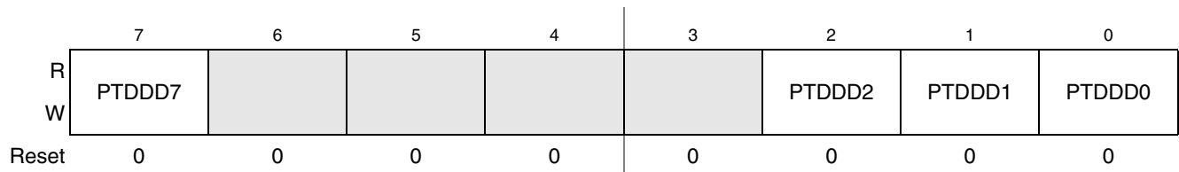
Figure 6-18. Data Direction for Port D (PTDDD)
