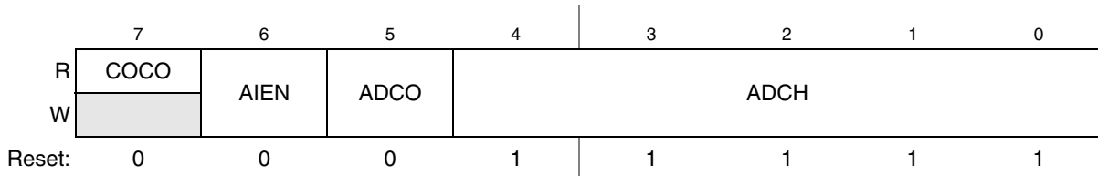
Figure 10-3. Status and Control Register (ADCSC1)
