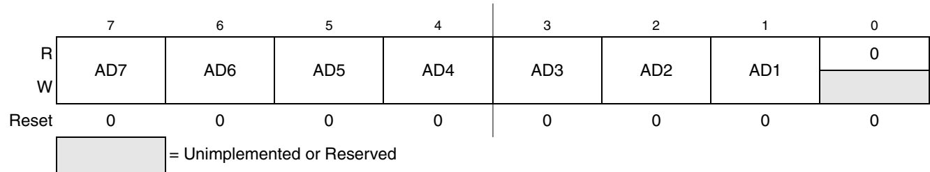
Figure 11-3. IIC Address Register (IICA)
