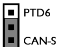
Figure 8-4: Can Operation Mode Selection (J6)
