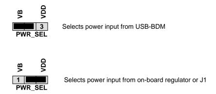
**NOTE:** Set PWR\_SEL jumper to VB during application development. Use barrel connector input (PWR) to support LIN functionality if needed.
