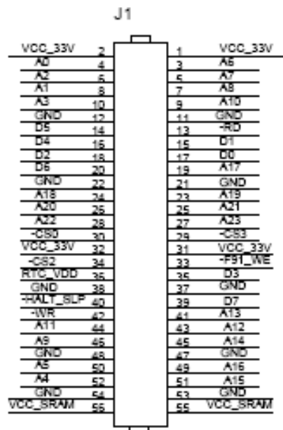
Figure 3. eZ80Acclaim! MDS Adapter Board Peripheral Bus Mini-Module Connector J1 Pin Configuration
