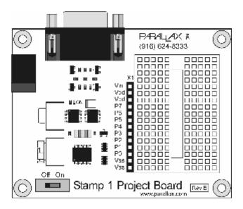
For permanent projects, you may leave off the breadboard and solder components directly to the PCB. Parallax offers a range of accessory component kits for the BS1 Project Board. The figure below shows the layout of the printed circuit board:
