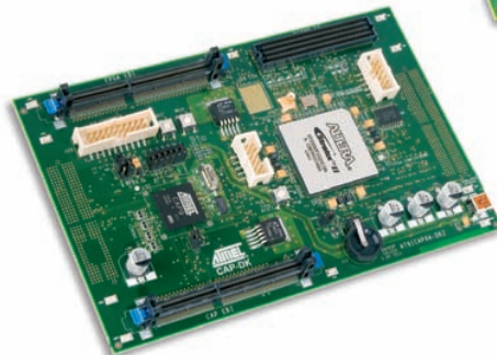
CAP9A Mezzanine Board
