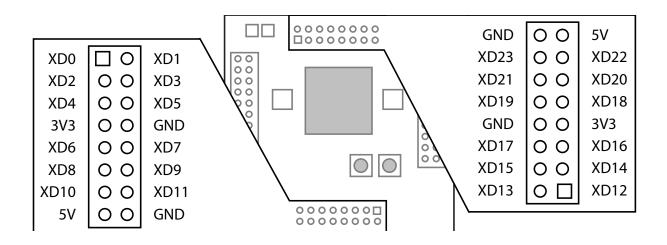
Each expansion header provides a bank of 12 I/O pins, which are mapped to the ports as described in the table on the next page, and four power/ground pins.
