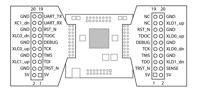
The XTAG-2 converts between XSYS and USB 2.0, allowing the XK-1 to be connected to most PCs. On power on, the XS1-L1 boots from the on-board flash memory. The XS1-L1 can then be put into JTAG mode by the PC, which then boots another program.
