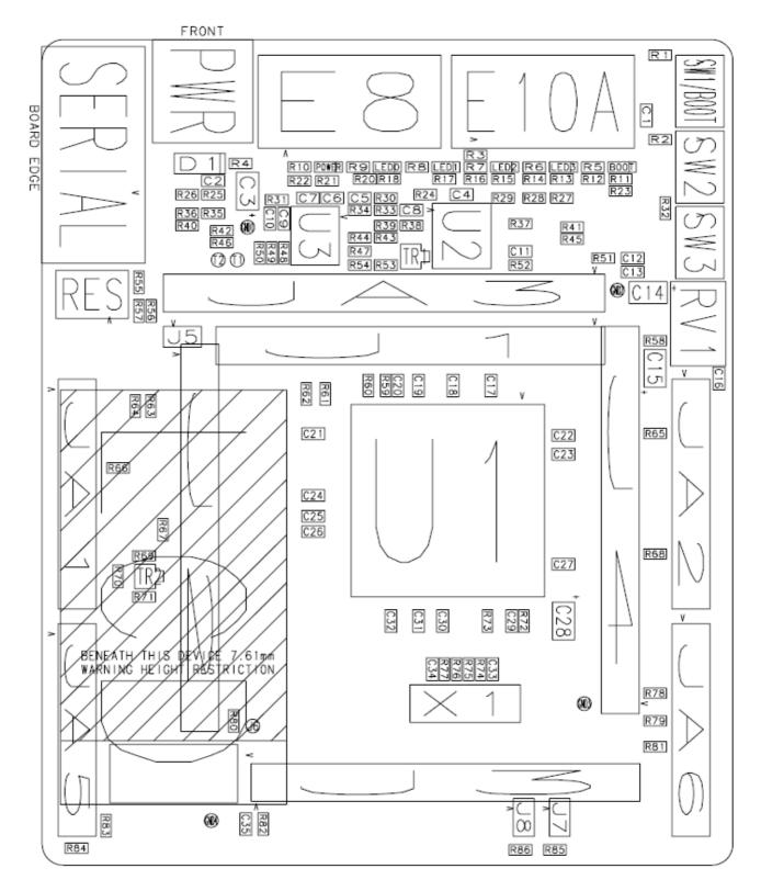
Figure 11-1: Component Placement (Top Layer)
