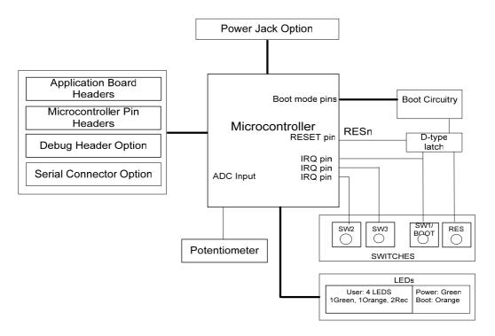
Figure 5-1: Block Diagram
