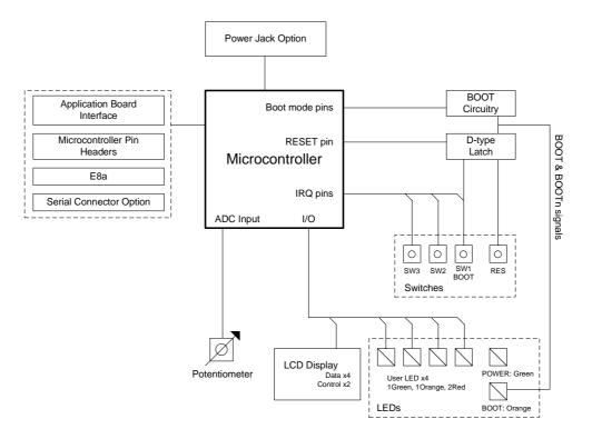
Figure 5-1: Block Diagram
