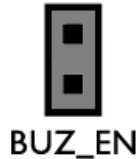
Figure 7-29: Piezo Buzzer BUZ_EN (J44)
