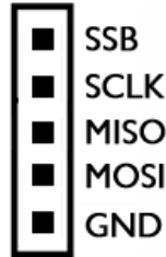
Figure 7-8: SPI Port Header
