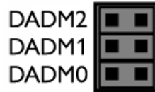
Figure 7-19: Differential Analog Channel Inputs Header DADMx (J29)
