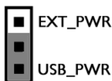
Figure 7-1: Power Source Selection Header (J3)
