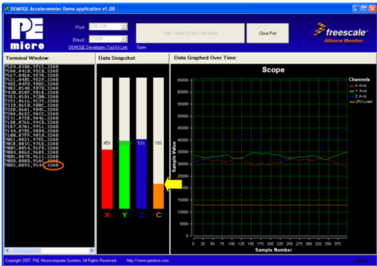
Figure 3-9: AccelerometerDemo running on 8-bit S08 QE128 in data averaging mode. Yellow arrow highlights the bus cycles required to average the last 16 readings of the 3 axes. Value shown in orange circle is the number of bus cycles in hex.
